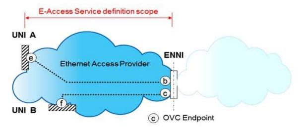
Figure 1. Scope of the E-Access Services Definition.
