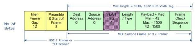
Figure 6. Length of an Ethernet frame as measured with and without the 20 byte inter-frame overhead.
