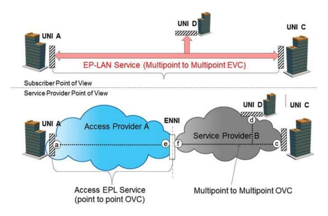
Figure 9. EP-LAN Service as implemented across two networks using Access EPL, showing the Subscriber and Service Provider Points of View.
