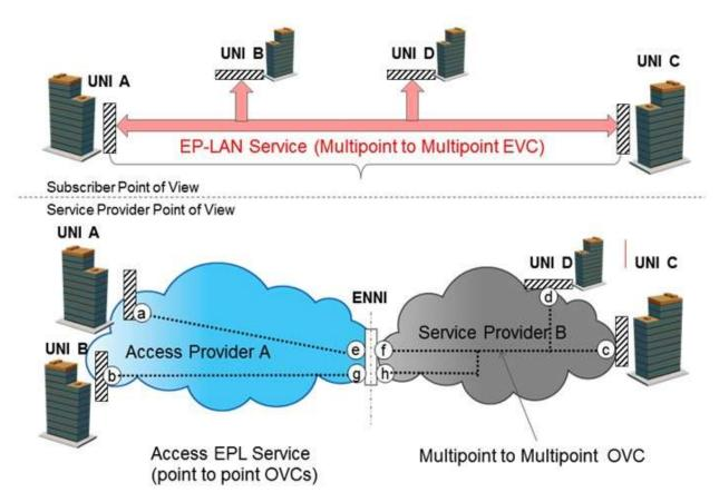
Figure 10. EP-LAN example illustrating a Service Provider using hairpin switching between UNI A & B.
